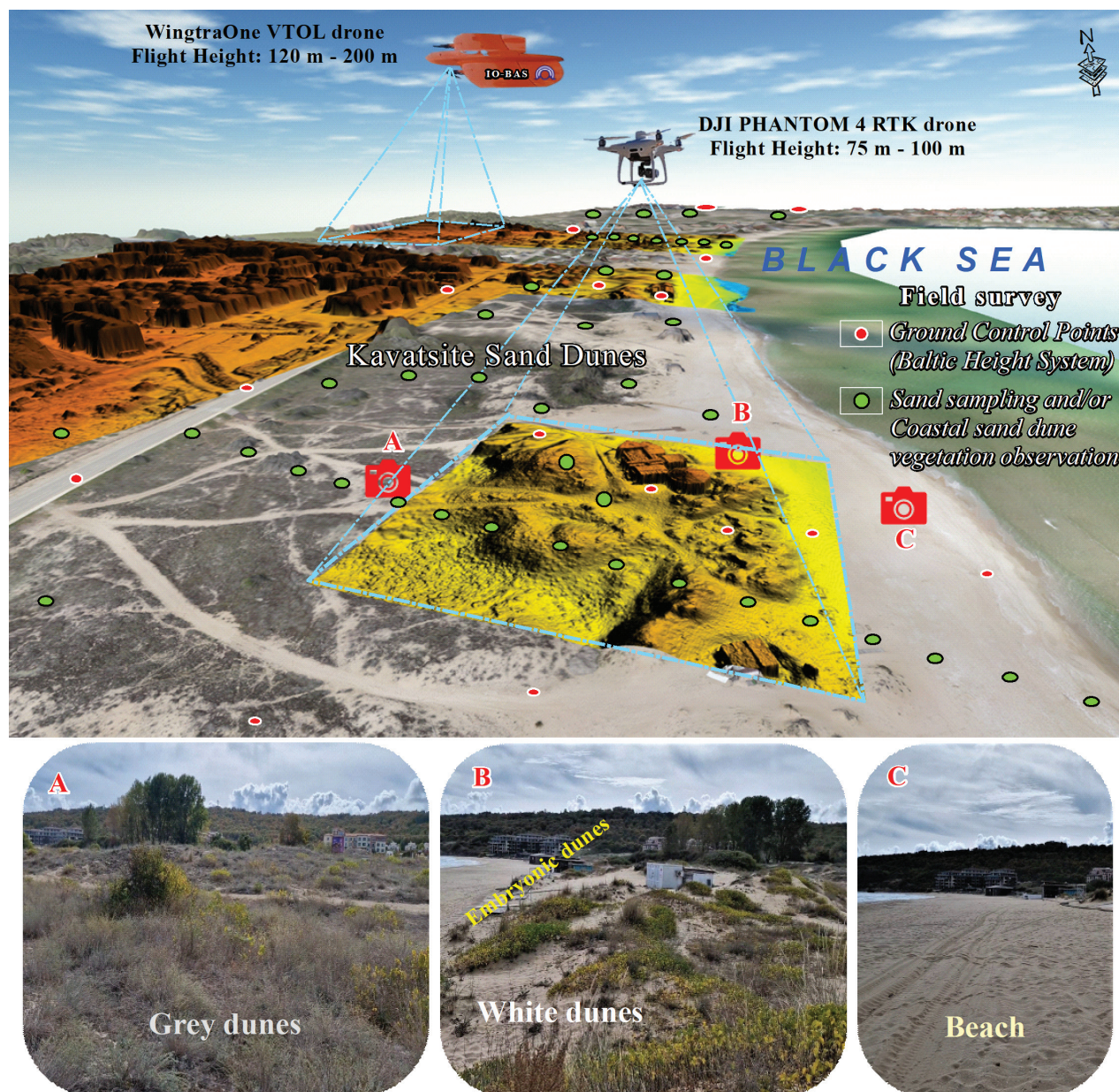
Figure 3. Example of field surveys and UAS mapping of coastal dune landforms using WingtraOne and DJI Phantom 4 RTK drones at Kavatsite-Smokini beach-dune system (Location on Fig. 4).
