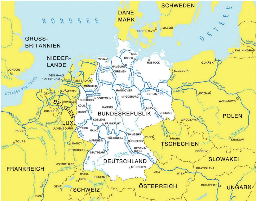
**Figure 2.** Overview of the system of German federal waterways within the Central European waterways network (Source: WSV).
