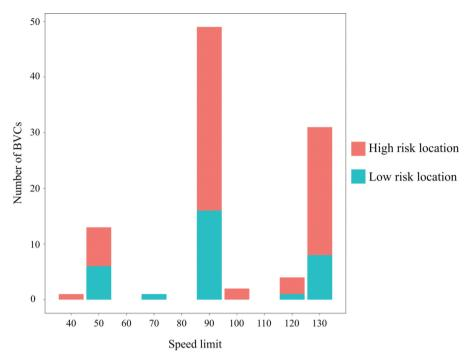
**Figure 4.** BVC counts across legal speed limits. Red indicates BVC counts in high-risk locations, where the collisions may have been unavoidable according to the sight distance set against the stopping distance, whereas blue marks BVC counts in low risk locations.
