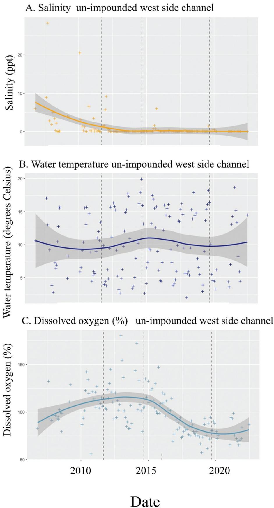
**Figure 5.** Water quality Elwha west un-impounded side channel 2008–2021. Hatched lines indicate dam removal phases left to right: dam removal beginning, dam removal ending, and five years after dam removals ended.
