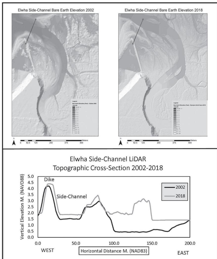
**Figure 4.** Elwha side-channel topography between 2002 and 2018 from bare earth LiDAR. LB = lateral bar.
